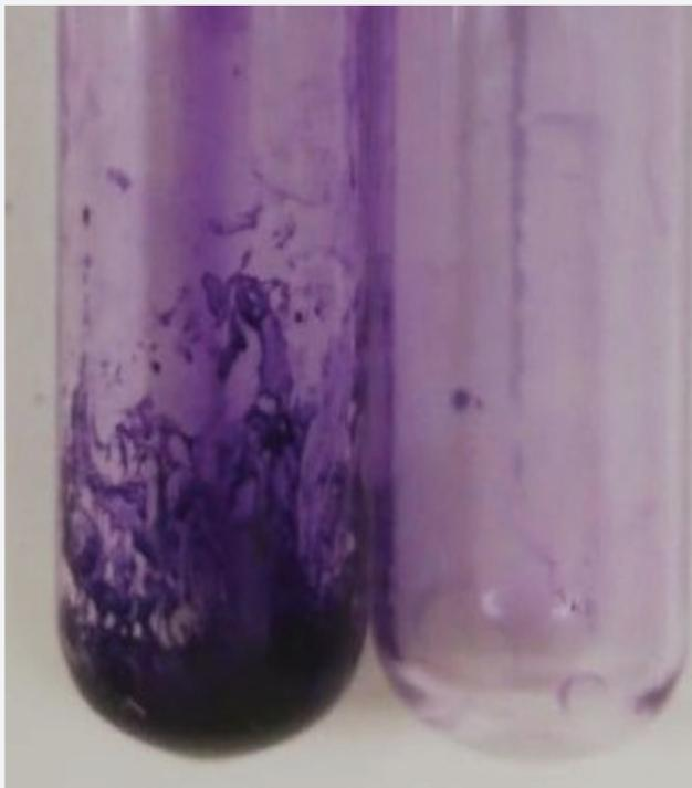
**Figure 2.** Biofilm production by Christensen et al.<sup>1</sup> standard tube method with SDB positive (left) and negative (right) glass tubes -close up photo-
